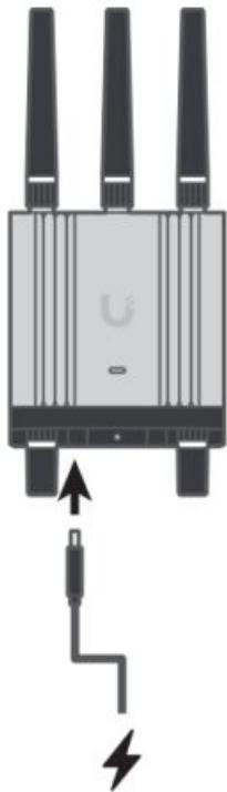
3. This equipment is provided with a detachable power cord which has an integral safety ground wire intended for connection to a grounded safety outlet.
