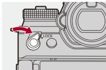
Aligning the operation lock lever with the [LOCK] position enables disabling of the operation parts set in [Lock Lever Setting] of the [Custom] ([Operation]) menu. (→[\[Lock Lever Setting\]: 674](#))
