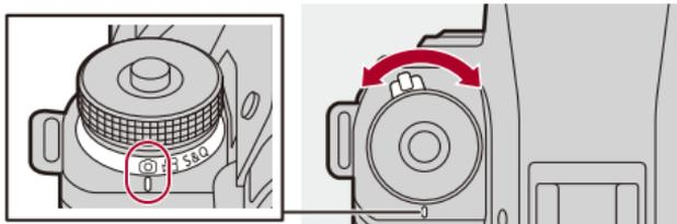
Use the mode dial to switch the recording mode.
