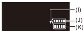
(I) USB connection cable supplying power
